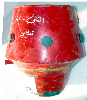
IRAQI NAVAL MINE, MOORED/DRIFTING, CONTACT, AL-MUTHENA/35
