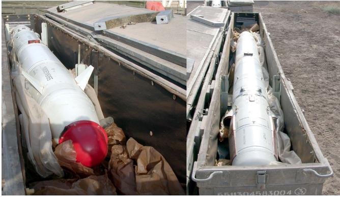
U.S.S.R. GUIDED MISSILE, AIR-TO-SURFACE, AS-12B (KEGLER)
