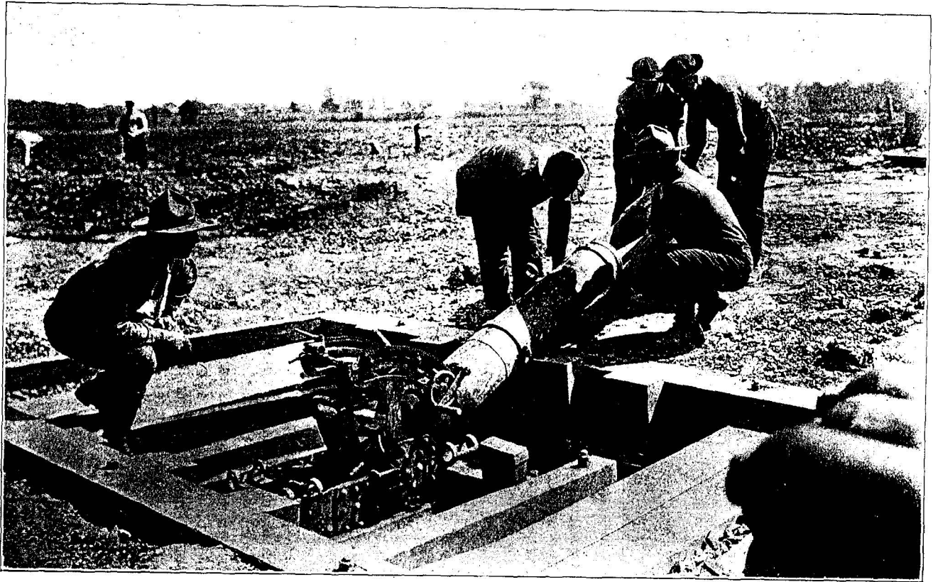
FIG. 102.—240-mm. trench mortar. Loading with projectiles. These are carried in a tray with handles.
